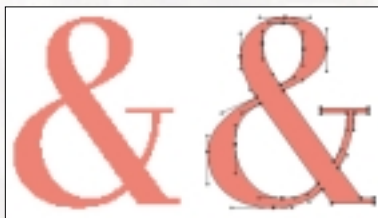
Left: images created in Photoshop are made from square pixels placed on a grid. Right: Illustrator graphics are made from paths, which allow them to always appear smooth when printed to a PostScript printer.
