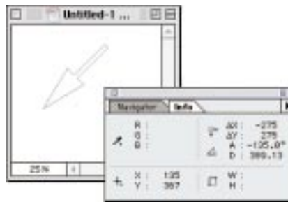
The Info palette will indicate the length (D) and angle (A) of the line being made.
